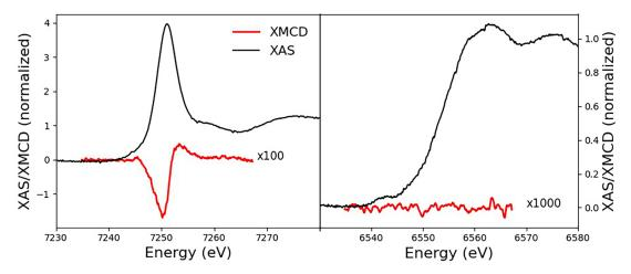
FIG. 7. X-ray absorption spectra and associated dichroic signal at Gd (left) and Mn (right) edge, performed at 1.3 T and 6 K. Dichroic signals are multiplied by a factor of 100 and 1000, respectively, for a sake of visibility.
