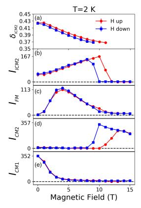
FIG. 6. Evolution as a function of the magnetic field along the b axis and T=2 K of the incommensurate position  $\delta$  of the  $q_{ICM2}=(\frac{3}{2},0,\delta)$  phase (a), its associated intensity  $I_{ICM2}$  (b), the intensity of the ferromagnetic contribution  $I_{FM}$  (c), the intensity  $I_{CM2}$  at  $q_{CM2}=(\frac{3}{2},0,\frac{1}{4})$  (d), and the  $q_{CM1}=(\frac{3}{2},0,0)$  intensity  $I_{CM1}$  (e).
