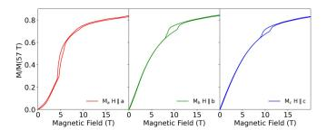
FIG. 1. Magnetization along the three different crystallographic axes as a function of magnetic field at  $T=2~\rm K$ . The lower curve corresponds to the increase in magnetic field strength, while the upper curve corresponds to its decrease.
