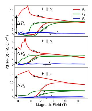
FIG. 3. Variation of the electric polarization along a, b, and c with respect to zero-field initial state as a function of increasing and decreasing magnetic field at 2 K.  $\Delta P_a$  at zero field after field cycling is indicated for each direction of the magnetic field. Its average among the three orientations is around  $10 \text{ nC/cm}^{-1}$ .
